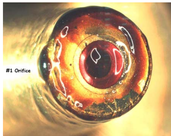
Figure 1: Varnish on Servo Orifice
