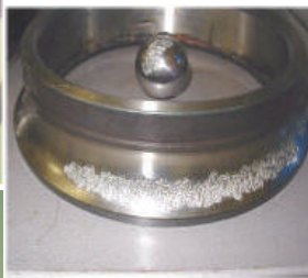
Spalling of inner race and rolling element
