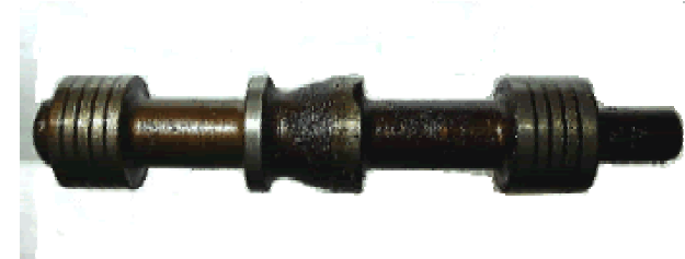
Varnish formation on spool valve
