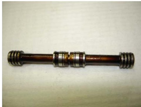
Varnish formation on spool valve
