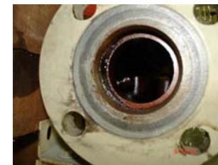
Varnish plated on heat exchangers
