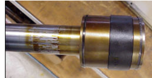
Varnish formation on Inlet Guide Vane
