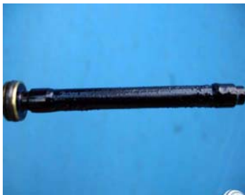
Varnish formation on pencil filter
