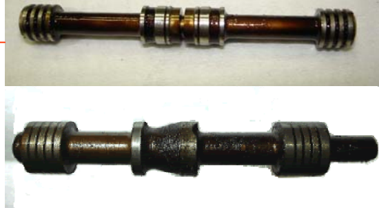
Varnish & sludge Problem Servo Valve Trip /fault due to valve sticking
